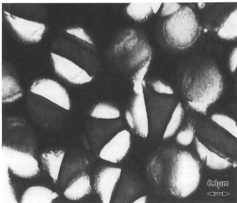
Figure 3. Transmission electron micrograph of composite latex particles of polystyrene (dark areas within particles) and poly(ethyl methacrylate) (light areas) stained with \text{RuO}_4 and phosphotungstic acid (21).
